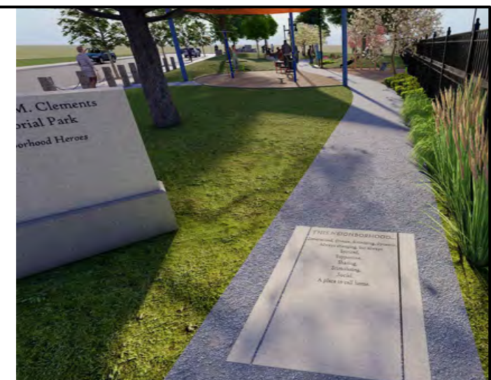
New W Clifford St entrance with granite fountain stone inset in semi-pervious stone dust paving
