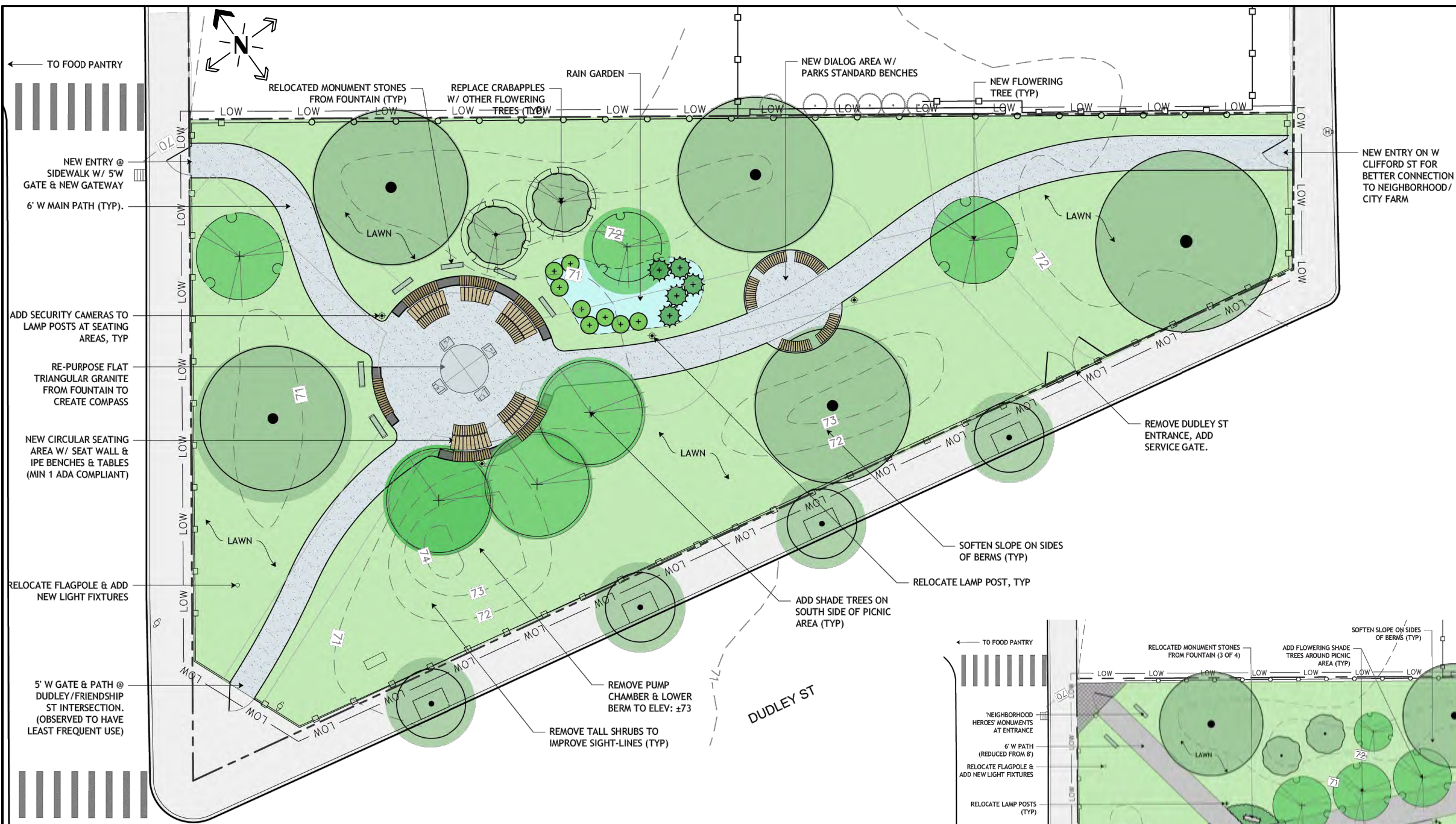
Clifford St Entrance from Concept A This design removes the existing 6' high wrought iron fence and replaces it with the city-standard 4' high welded-wire mesh, surrounding the whole park, including previously unused space along Clifford St.
