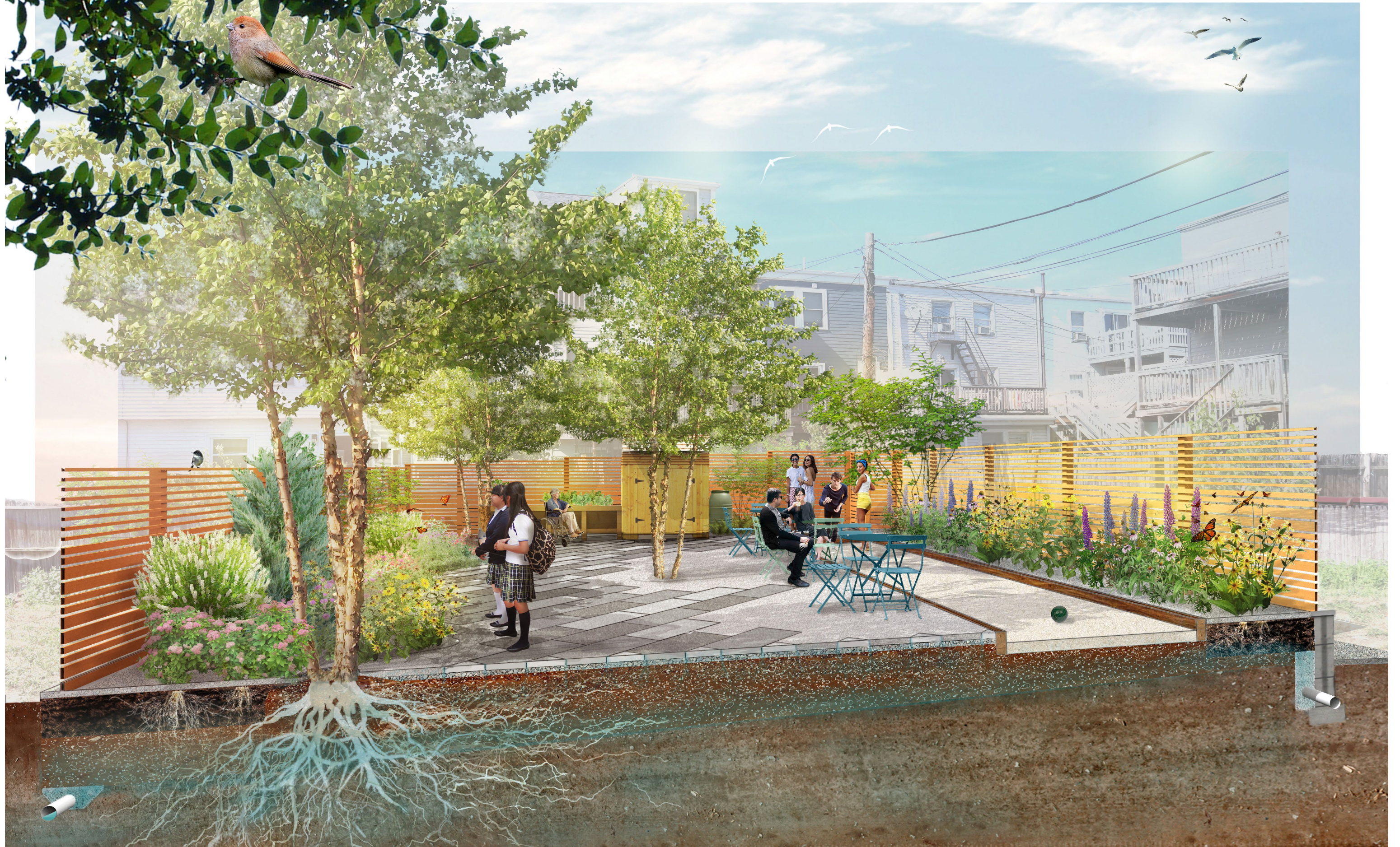
Section-perspective view revealing stormwater flowing through permeable paving and plant roots spreading out inside sand-based structural soil.
