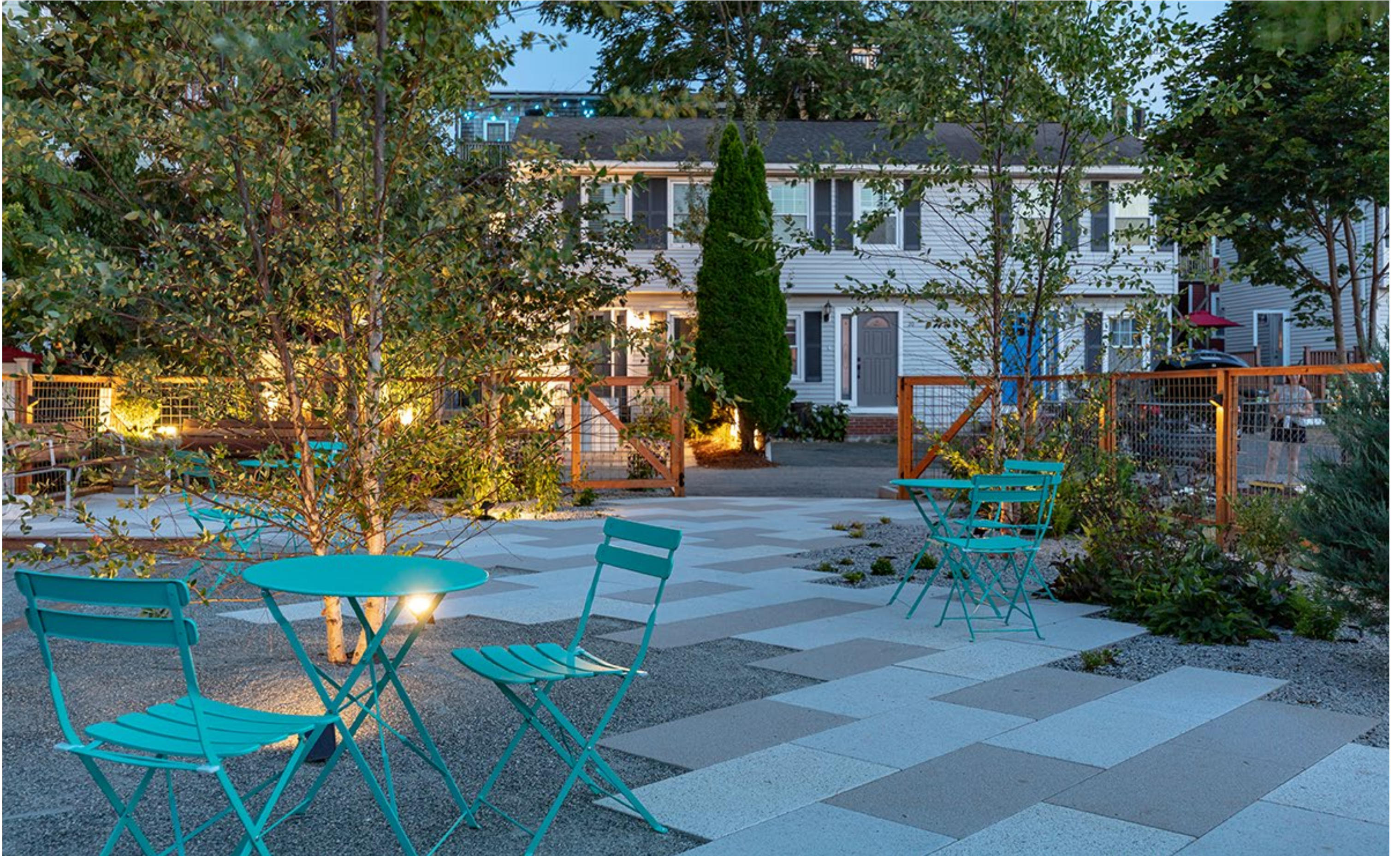
Movable and colorful bistro sets sit atop a permeable surface of oversized pavers with 1/8" open joints, decomposed granite, and planting beds. The fence panels are a simple cedar and hogwire system that allows for visual porosity and lower costs in a time of extreme material shortages.
